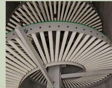
We have also embraced passive energy-saving solutions. In select production lines, power-driven material conveyors have been replaced with gravity-fed flow chutes, reducing electricity use and simplifying maintenance aligned with our lean and green manufacturing philosophy.
